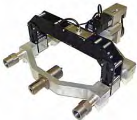
Fig. 3. Exterior of the Welding Manipulator with AQCS
